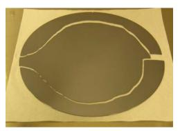
Fig 1. Catastrophic fracture of a 200mm diameter silicon wafer
