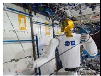
Fig 2: Robonaut 2 – the first dexterous humanoid robot in space – is pictured on ISS. Credit NASA
