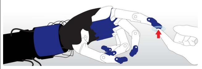
Fig 3:Tactile human-machine interface with QTC skin developed for robotics with NASA and MIT
