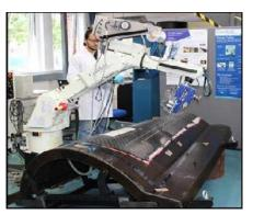
Figure 3: Tufting robot at Cranfield inserting tufts in a double-curvature surface.
