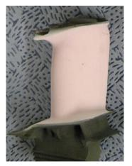
Figure 1: An aerofoil coated with a low K thermal barrier doped with Erbia at Cranfield
