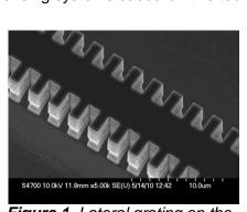
**Figure 1.** Lateral grating on the side wall of a QCL.
