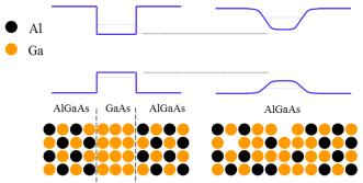
**Figure**: Illustration of band-structure and layer structure of a non-processed (left) vs. a QWI processed quantum well (right)
