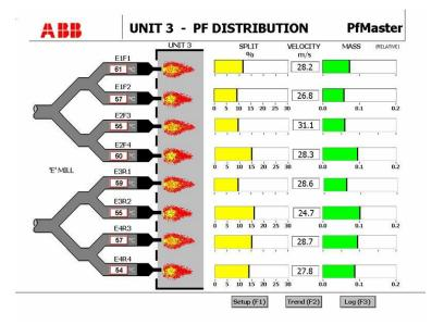
ABB PfMaster control system for efficient balancing of split fuel flows for power station boilers, based on original Teesside research.
