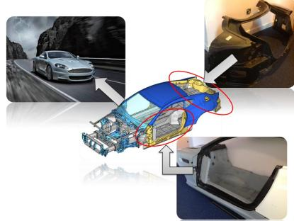
Figure 1: showing carbon fibre parts manufactured using DCFP and their location on the automobile
