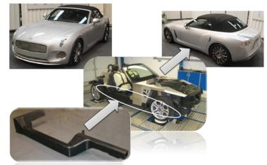
Figure 2: carbon fibre chassis rails manufactured using the Raycell concept and its location on the Bentley T35 demonstration vehicle
