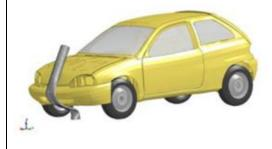
design guide for passively safe hybrid composite posts. The design guide aims to enable evaluation of the feasibility of variations in the design of the composite post against the European Standard EN12767 limits for ASI (Acceleration Severity Index) and THIV (Theoretical Impact Velocity). The design parameters investigated included: Number of carbon tows; Layup variation; Wall thickness variation; Post diameter; Foundation type (granular sub base, sand, concrete).
