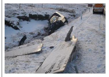
On the 4th December 2012 in icy conditions there was an accident on the A970 on the Shetland Islands. A vehicle struck one post of a two post Frangible Safety Post installation and the driver walked away unscathed. It is likely that should the vehicle have struck a traditional steel post installation the driver would have suffered significant injuries. The Frangible Safety Post that was struck performed and reacted exactly as intended through our patented design. [4.4]
