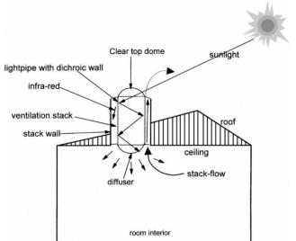
Figure 1: Illustration of Sola-Vent concept
