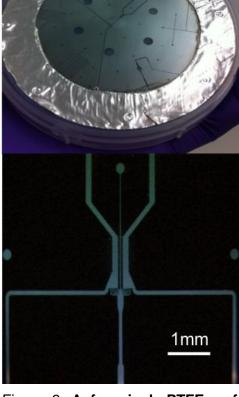
*Figure 3:* **A four inch PTFE wafer**, with a metal mask, showing deepetched microfluidic ducts (top). Fine detail of the microfluidic duct system on this wafer is also shown (bottom).
