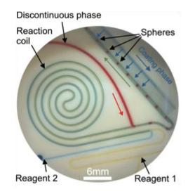
*Figure 1*: **Microsphere production chip**. Reagents 1 and 2 are precision delivered through flat capillaries, in which they are incubated within a reaction coil. After this they are interfaced with an immiscible discontinuous phase, thus causing the formation of droplet microspheres, which are then coated.
