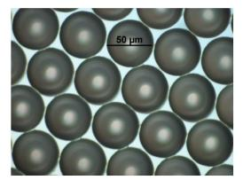
*Figure 2*: **Polymeric microspheres**, with a highly uniform diameter of 50 microns.
