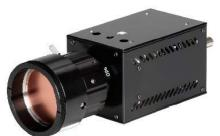
The Soltec THz Imager (IRV-TF083) [5.7]. Product IRV-TF030, built and mounted by the AIG, can be seen as the front coppercoloured element of the camera.
