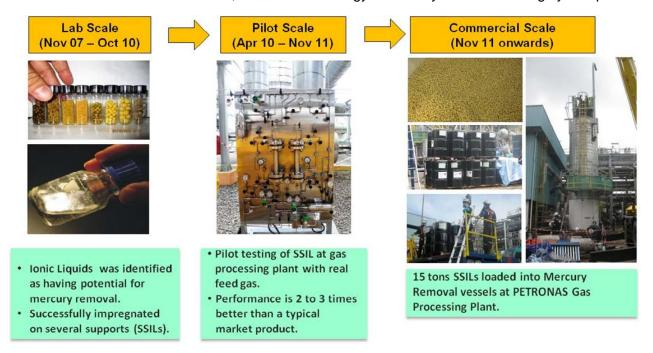
**Figure 1** Development of the mercury capture technology for natural gas clean up in conjunction with PETRONAS
