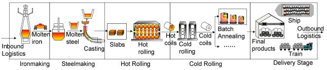
Figure 1. Stages of steel production and logistics system
