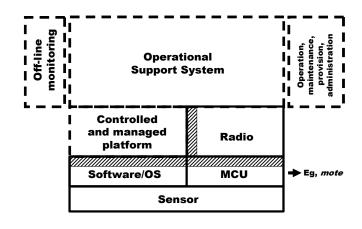
Figure 1: The four layers of the UCL system: (i) sensor components, (ii) the software, operating system and microcontroller unit (MCU); (iii) radio and network control and management system; and (iv) the operational support system, administration, provision and maintenance. Layers (iii) and (iv) together comprise an Integrated Service Layer (ISL).
