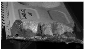
Fig 1 Runway debris damage to the leading edge of an undercarridge door of a transport aircraft
