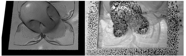
Figure 1: Ballistic impact into Dyneema armour panels at 1km/s with 60g copper projectile. Left: Improved numerical predictions; Right: Experimental test (from Figure 2 test).
