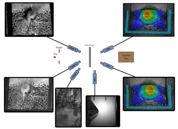
Figure 2: Enhanced ballistic testing of high performance composites
