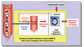
ABB's BoilerMax Nonlinear MPC for drum-boiler control
