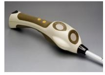
**Figure 1** The *UltraCane* handle showing ultrasonic sensors and feedback buttons.
